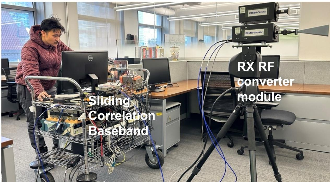
Indoor radio propagation measurements at 16.95 GHz.
