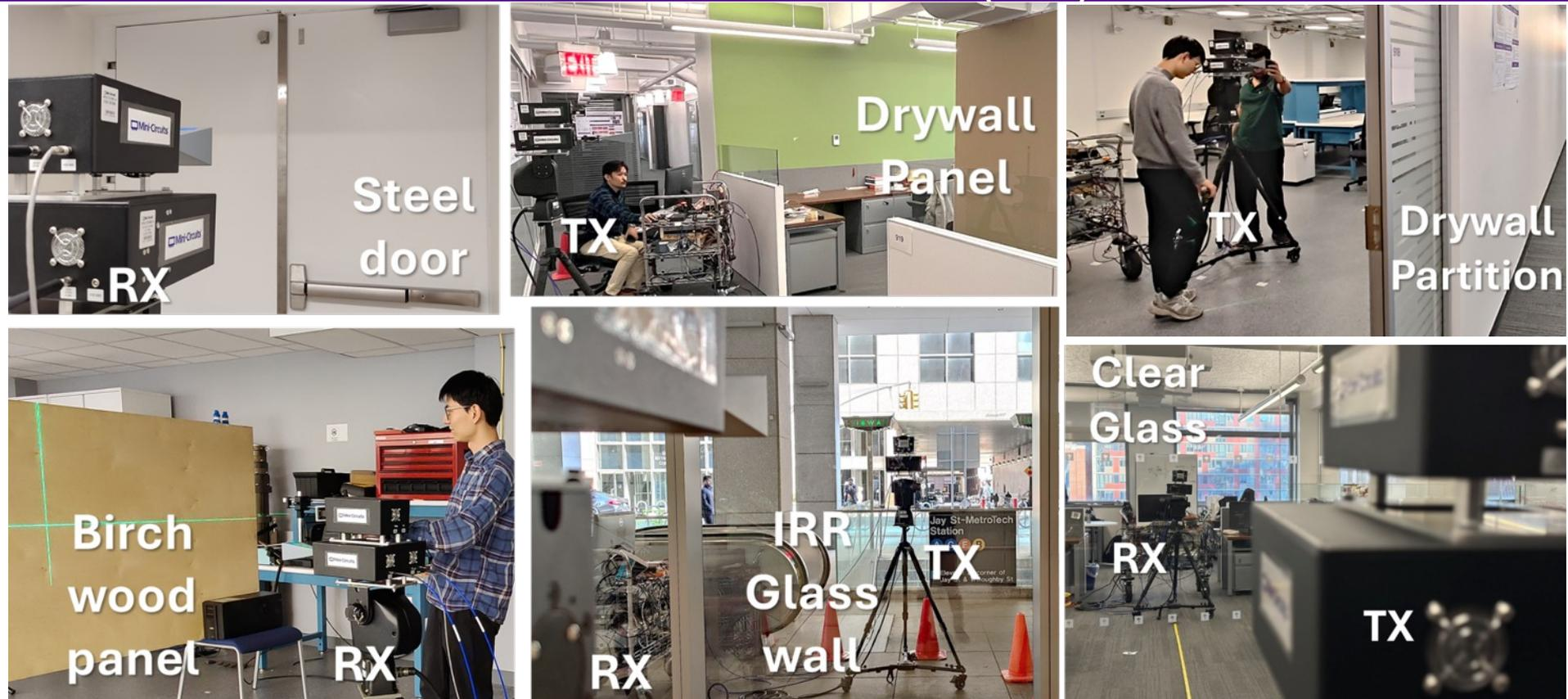
Fig. Different materials measured for penetration loss
