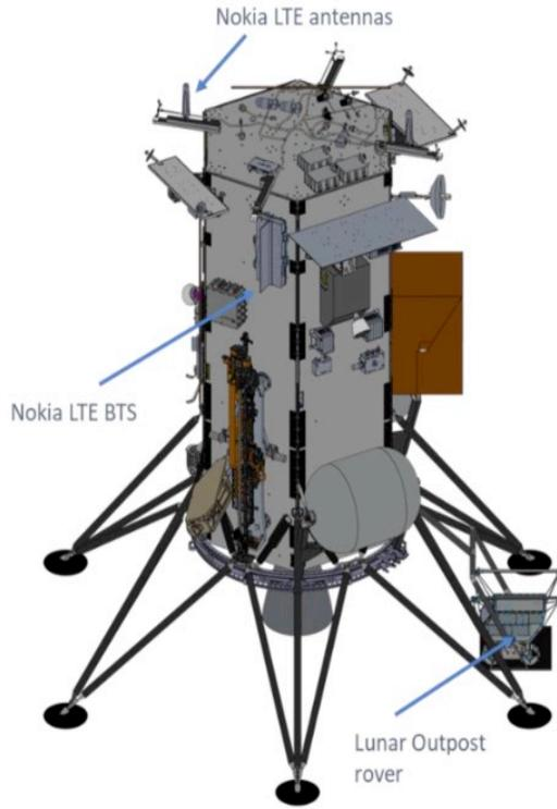
Figure 1. Intuitive Machines lander with Nokia LTE BTS and Lunar Outpost rover (stowed configuration)
