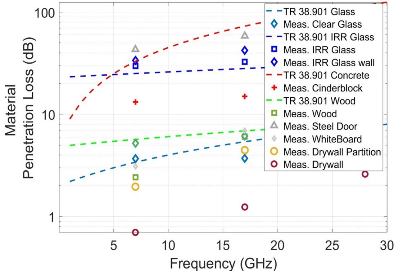
Comparison of measured material penetrations with 3GPP standard material penetration loss curves [1], [2]
