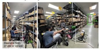
Fig. 3: Photos taken from Factory C. The TX was set at 2.5 m, and the RX was set at 1.5 m and 0.5 m.
