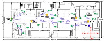
Fig. 1: TX and RX locations in Factory A. Six TX locations are denoted as stars, and 17 RX locations are denoted as circles, resulting in 27 TX-RX location pairs for channel measurements.
