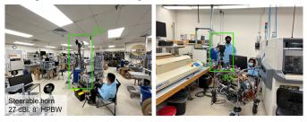
Fig. 2: Photos taken from Factory B. The TX was set at 2.5 m, and the RX was set at 1.5 m.
