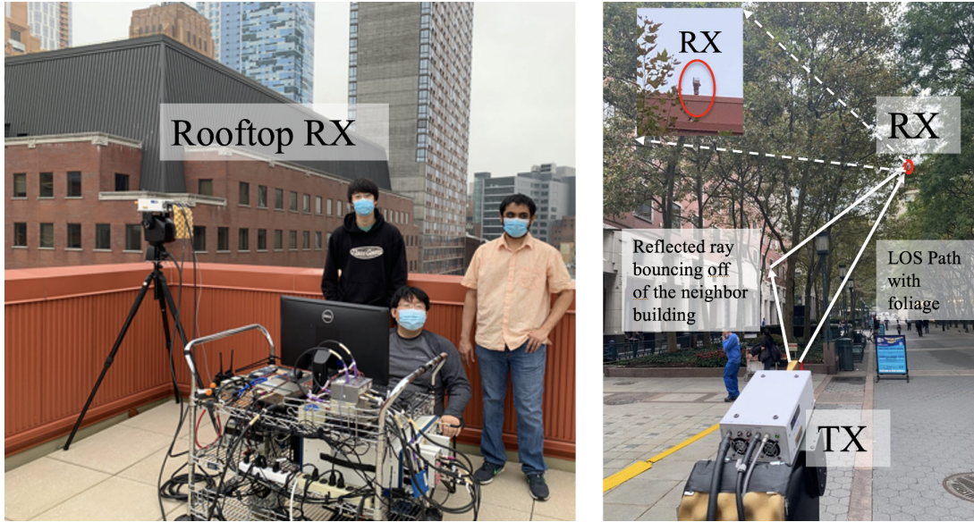
Figure 5.3: The RX is at heights of 1.5 m above the roof corner, which prevents the RX from being shadowed by the railing boundary, emulating a passive receiver in a satellite. The TXs are at heights of 1.5 m above ground working as mobile terminals [67].
