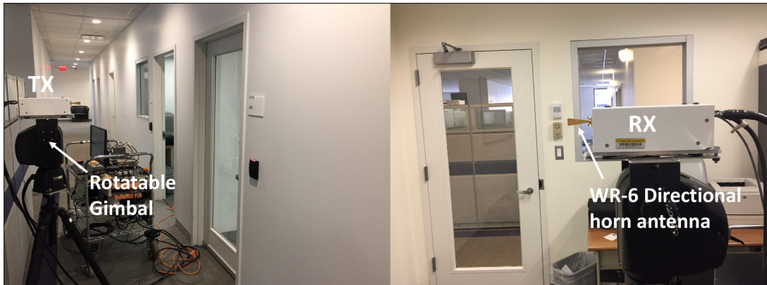
Figure 2.3: 140 GHz channel sounder with directional horn antennas.
