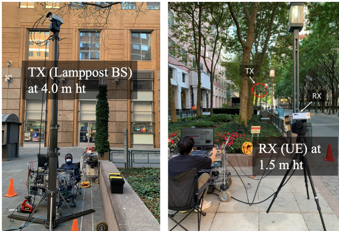
Figure 4.5: The 142 GHz channel sounder system and outdoor UMi measurements in NYU courtyard in Brooklyn, with the TX antenna at 4.0 m above ground level to emulate outdoor small-cell lamppost base stations (BS) and the RX antenna positioned 1.5 m above ground level, similar to the height of a handset terminal [67].
