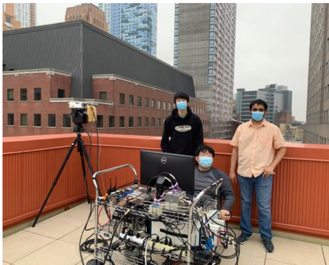
RX on the roof, emulating a passive receiver at the satellite, search every direction to capture any signal
