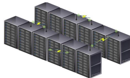
Short-range THz wireless connectivity in data centers [2]
