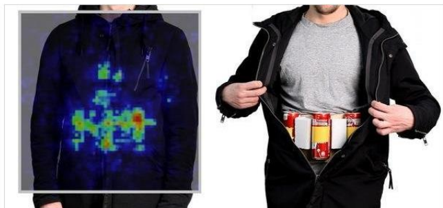
Body scanner using THz imaging to detect explosives [1]
