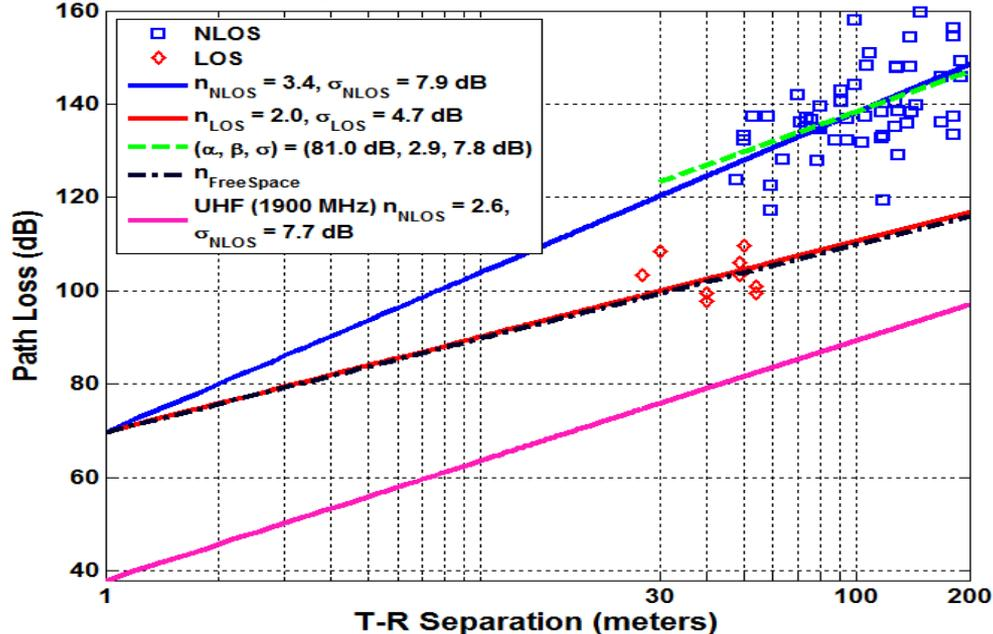
$PL_0$  is path loss measured at close-in distance  $d_0$
