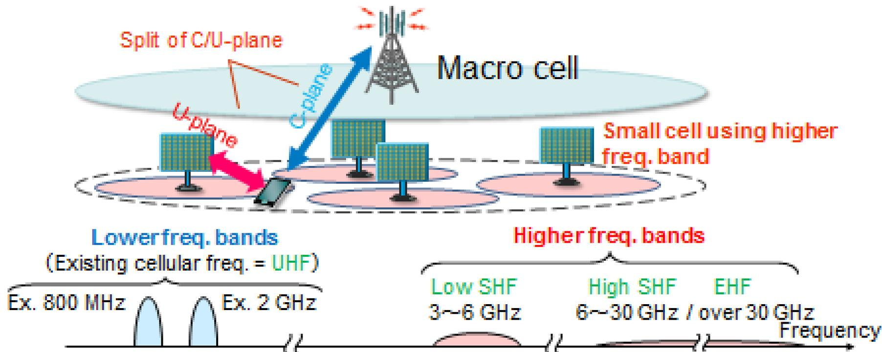
**Phantom Cell concept can easily exploit higher freq. bands!**
