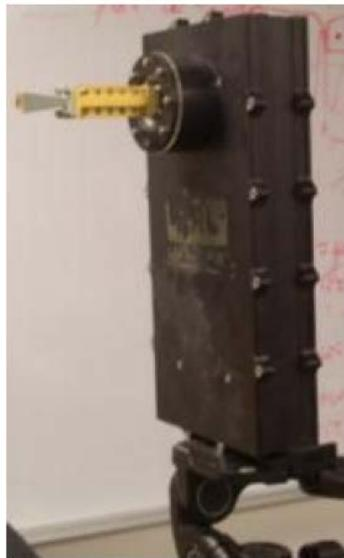
Upconverter and Downconverter assemblies at 38 and 60 GHz, newer ones built at 28 GHz, 72 GHz
