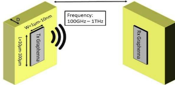
On-chip & chip to chip Terahertz communication links [20]
