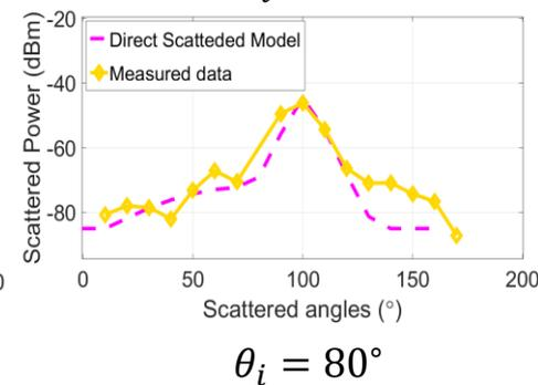
Comparison between measured data and the dual-lobe Directive Scattering (DS) model at 142 GHz [1,26].
