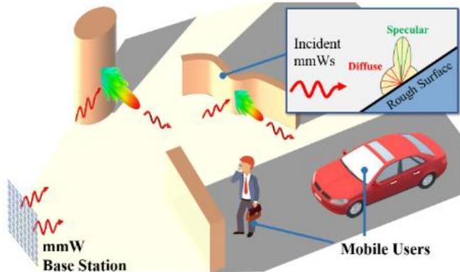
mmWave imaging and communications for Simultaneous Localization And Mapping (SLAM) exploiting the scattering properties at mmWave [18]
