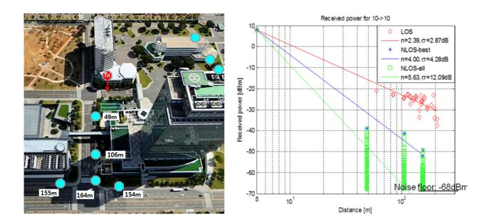
The results obtained from the three measurement campaigns in 28/38 GHz bands, show that pathloss exponent in NLoS link is between 3.2 and 4.58. This range is not much discrepant from that in the conventional IMT bands (i.e. 3.67~3.91) [17].
