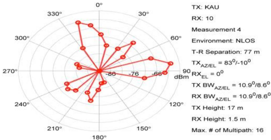
Signals arrive within 2 to 5 “lobes” in NYC over many azimuth angles in Non Line of Sight (NLOS)
