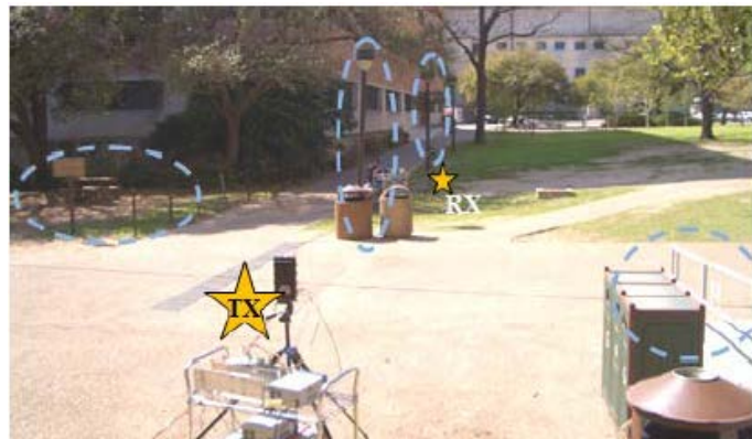
Figure 5 Photo of campus measurement location with surrounding buildings, trees, light posts, and handrails. Metallic objects were found to be useful reflectors that can be exploited in non-LOS conditions (circled in photo) [7].
