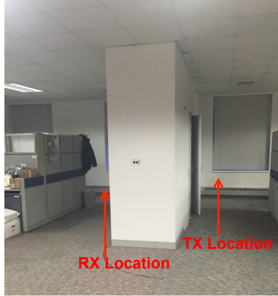
FIGURE 4.8: TX and RX locations for indoor corner measurements in the NYU WIRELESS research center on the 9 th floor of 2 MetroTech Center. The material of the corner is drywall.
