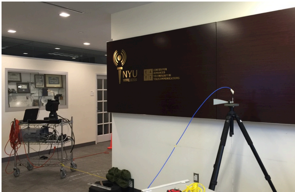
FIGURE 4.23: Indoor wooden corner diffraction measurements at 26 GHz.
