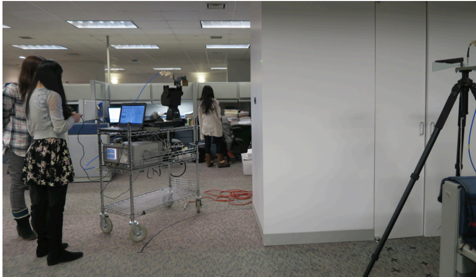
FIGURE 4.22: Indoor drywall corner diffraction measurements at 26 GHz.
