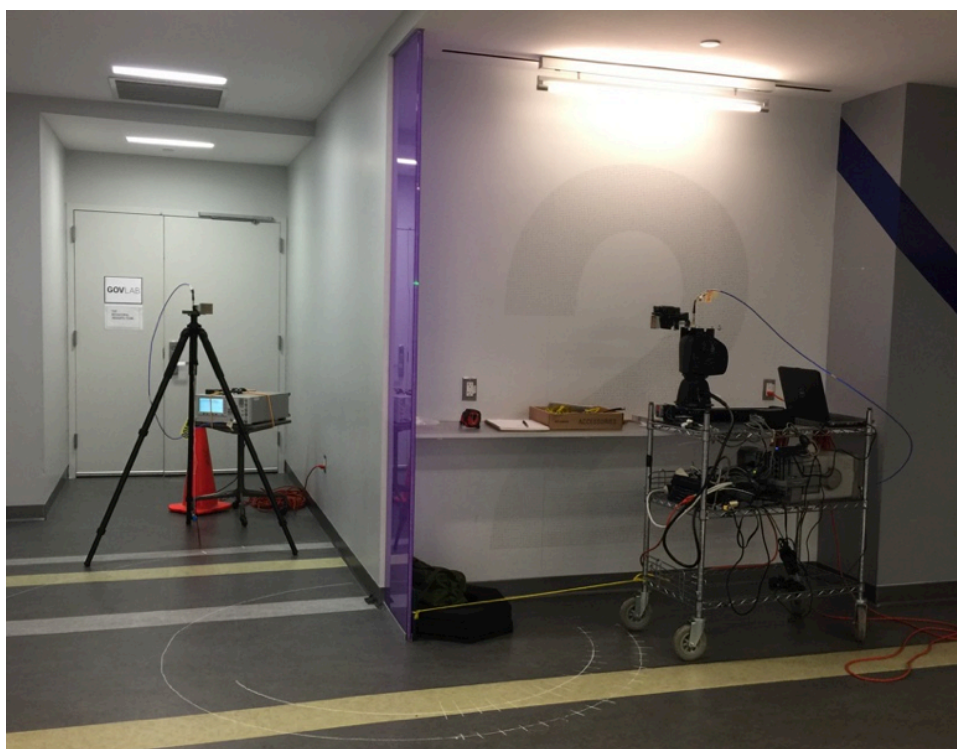
FIGURE 4.25: Indoor plastic board diffraction measurements at 26 GHz.
