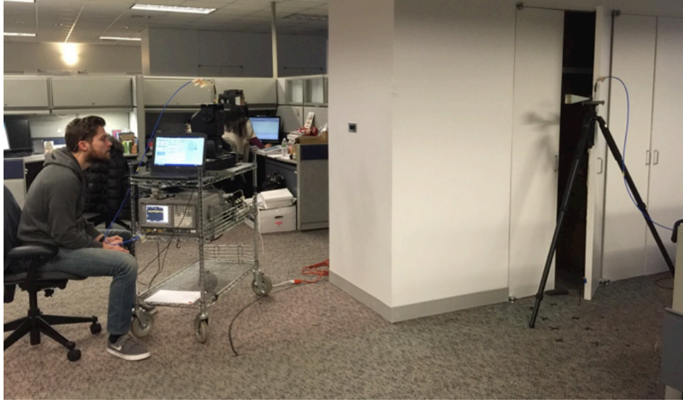
FIGURE 4.21: Indoor drywall corner diffraction measurements at 26 GHz.
