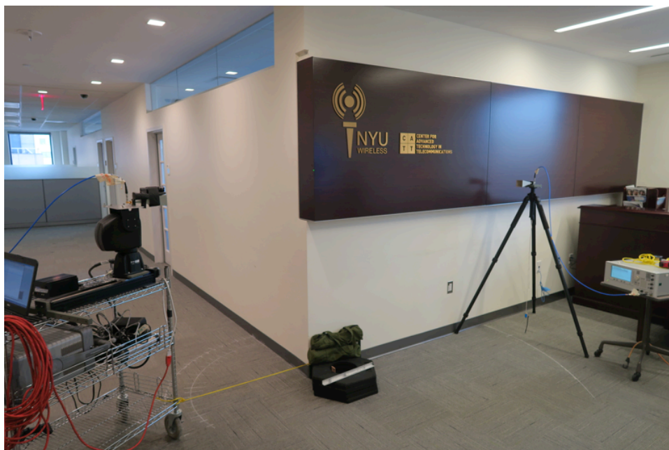
FIGURE 4.24: Indoor wooden diffraction measurements at 26 GHz.
