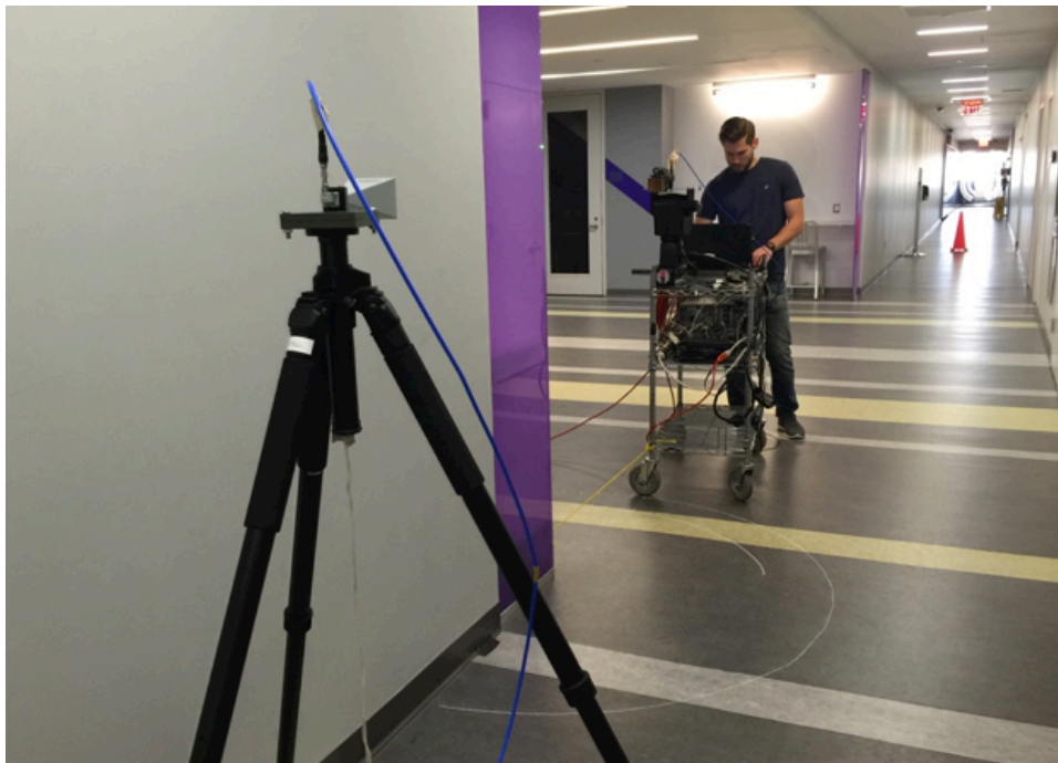
FIGURE 4.26: Indoor plastic board diffraction measurements at 26 GHz.
