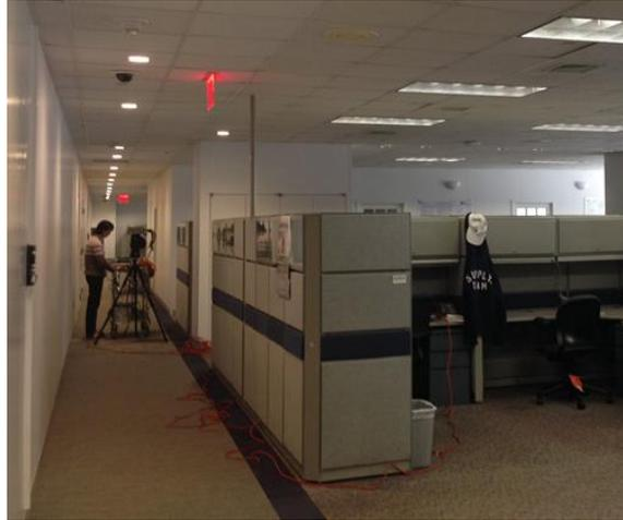
Fig. 3.17 Receiver location for one of the MTC1 TX site measurements with the antenna attached to the down-converter box that is mounted on top of a steerable gimbal that is mounted on top of a tripod to reach a height of 1.5 meters.
