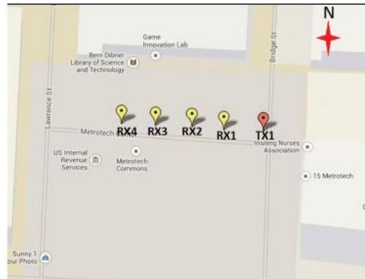
Fig. 3.23 Map of the TX and RX locations for the outdoor foliage and ground bounce measurements. The T-R separation distance between TX1 and RX1 is 10 meters, and an additional 10 meters separation exists for each subsequent RX location. The foliage type is cherry trees with leaves and flower blossoms.
