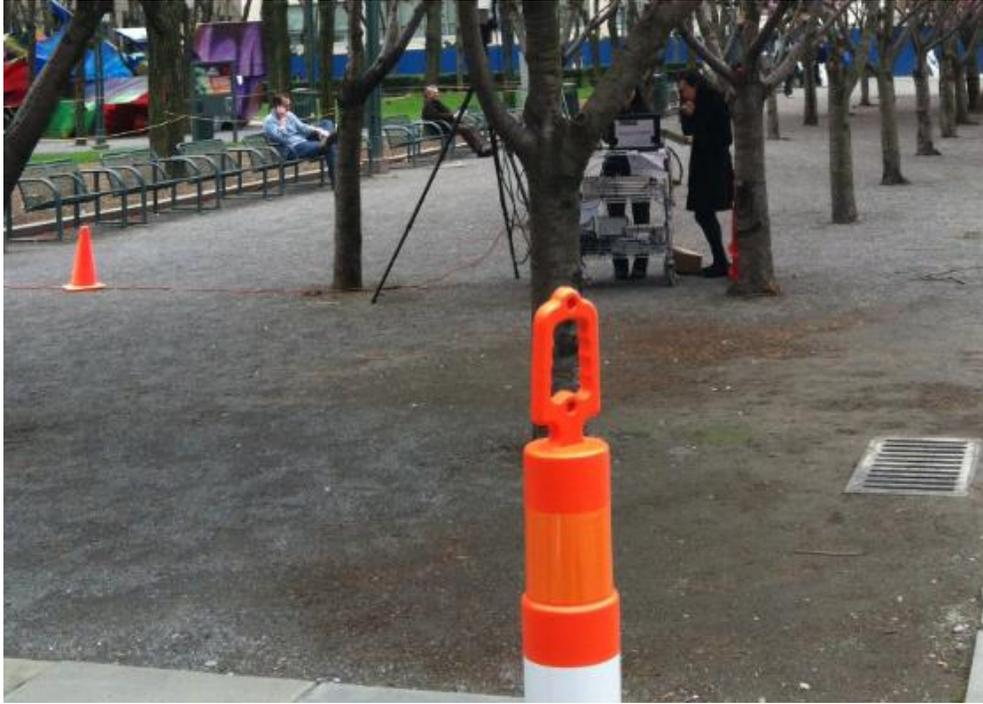
Fig. 3.21 Photo of the foliage measurement ground bounce surface (soil / dirt / gravel) at the MetroTech Commons Courtyard, located between the trees and beneath the branch canopy.
