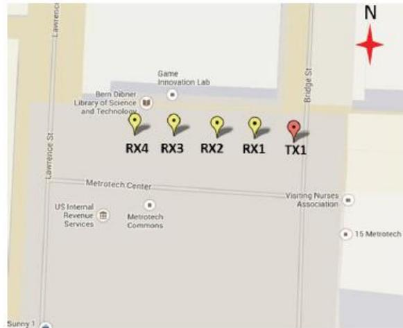
Fig. 3.22 Map of the TX and RX locations for the outdoor free space measurements. The T-R separation distance between TX1 and RX1 is 10 meters, and an additional 10 meters separation exists for each subsequent RX location.
