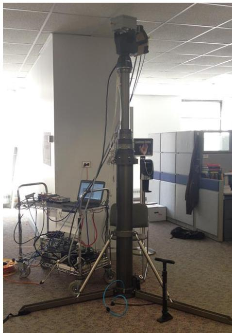
Fig. 3.16 Transmitter located at the indoor MTC1 location with the antenna attached to the up-converter box that is mounted on top of a steerable gimbal, which is mounted on top of a pneumatic mast to reach the height of 2.5 meters.
