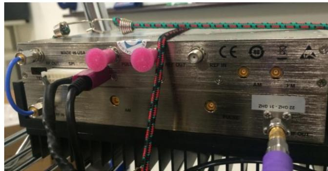
Fig. 3.4 Phase Matrix QuickSyn frequency synthesizer for the LO signal. The top box is a model FSW-0020 digital frequency synthesizer and the bottom box contains a frequency doubler and amplifier.
