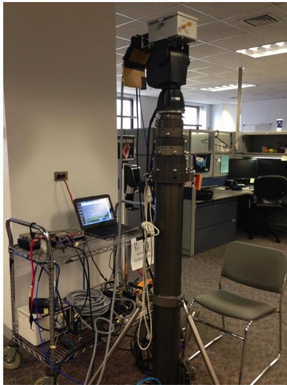
Fig. 3.8 Transmitter setup for the antenna pattern measurements. The height of the transmit antenna is 2 meters relative to ground.
