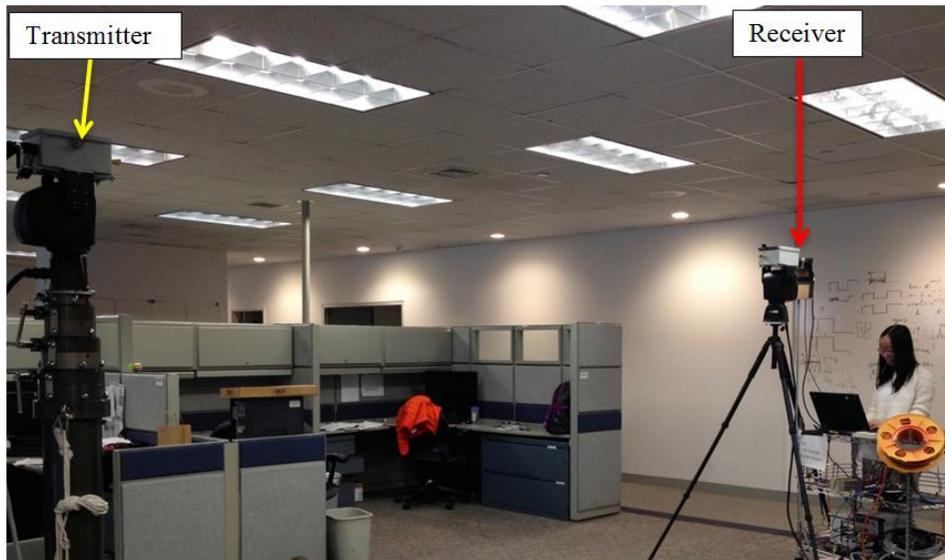
Fig. 3.10 Antenna pattern measurement environment. The majority of surrounding furniture was at a height lower than the TX and RX antennas.
