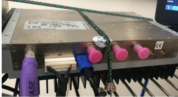
Fig. 3.3 Phase Matrix QuickSyn frequency synthesizer for the IF.
