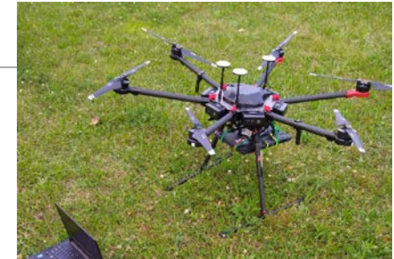
DJI Matrice 600 Pro (payload 6 Kg)
